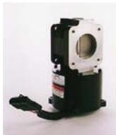
**The Flo-Tech™** integrated actuator/butterfly valve body is designed for direct replacement of conventional turbocharger bypass valve with actuator and linkage. The valve body will provide equivalent maximum flow rates of standard butterfly valve bodies of the same diameter. The Flo-Tech integrated actuator/valve body requires no actuator or linkage.
