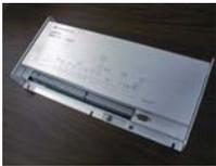
The **2301D and 2301D-EC Digital Load Sharing and Speed Controls** are used in electric generator systems for which load sharing is desired. They can be used with diesel or gas engines, or steam or gas turbines. The control utilizes a digital based speed control and provides a single serial port for PC communications. The digital design eliminates the use of potentiometers for tuning and load control.
