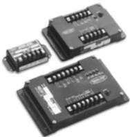
**ESS electronic speed switches** are used to protect against overspeed and underspeed, to detect starting speed and disconnect the cranking motor, to detect other critical speeds. These fully electronic switches can be applied to generator sets, starter motors, engines, conveyors, bus doors, PTO protection, magnetic brake retarders, transmissions, .... They can receive inputs from magnetic pickups, alternator output, ignition output, or the Mini-Gen® signal generator.
