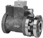
**The Gas Shutoff Valve** is designed to provide extremely fast shutoff to gaseous flow and to be used for emergency and normal shutdown operation. The valve operates at pressures up to 900 psia and its all stainless steel construction assures availability of the valve under all operating conditions. The valve design allows minimum pressure drop by utilizing a straight through flow, this also keeps all critical moving parts and seals out of the flow stream.
