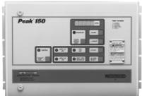
**The Peak® 150** digital control is designed to control a steam turbine driving a mechanical load. It provides tight control of speed (NEMA D) and includes an input for a 4–20 mA remote speed control signal, which can be used for a process-generated input to control the speed setting. Other features include dual speed control dynamics and overspeed trip test capabilities.
