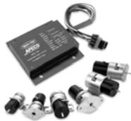
**APECS® actuators** work with APECS controls to provide proportional fuel control for construction, industrial, and agricultural equipment. Actuators are available with push or pull actuation, flange or base mount, 12 or 24 Vdc. Actuators come in 1.75" (44.5 mm), 2.50" (63.5 mm) and 3.00" (76.2 mm) diameter.
