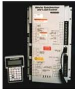
The **MSLC** control is a microprocessor-based load control designed for three-phase electric power generation sites equipped with Woodward DSLC Digital Synchronizer and Load Control units which operate in parallel with the utility. The MSLC is a synchronizer, a utility load sensor, an import/export load level control, a power factor control, and a master process control.
