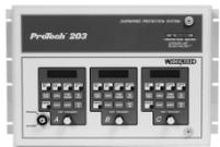
**The ProTech® 203** Overspeed Protection System monitors three individual magnetic pickups (MPUs) to provide overspeed protection for steam and gas turbines and other prime movers. The system replaces mechanical overspeed devices, especially in high-speed applications (above 10,000 rpm) when a mechanical overspeed device becomes unreliable.
