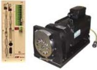
The **EM-80 and EM-300 gear-motor actuators** are intended to be mounted on large diesel, gas, and gasoline engines, and on all types of turbines, to control the position of engine fuel racks, turbine fuel valves, turbine and turbocharger variable geometry, and to handle timing control. These systems are well suited for engines without a mechanical drive or hydraulic oil supply.
