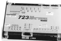
**The 723 Plus Digital Control** manages and controls reciprocating engines (gas, diesel, or dual fuel) used in power generation, marine propulsion, and gas compression/distribution. The control may also be used in cogeneration, power transmission/distribution, process management, pipeline pump stations, utility power generation, emergency standby power, and remote control station operation. The 723 Plus provides state-of-the-art control for new and retrofit situations.
