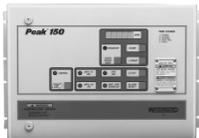
**The Peak® 150** digital control is designed to control a steam turbine driving a mechanical load. It provides tight control of speed (NEMA D) and includes an input for a 4–20 mA remote speed control signal, which can be used for a process-generated input to control the speed setting. Other features include dual speed control dynamics and overspeed trip test capabilities.
