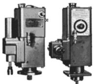
**The PG Dial and Lever governors** control the speed of diesel, gas, and dual-fuel engines in a variety of fields. Their applications include engines driving pumps, compressors, alternators, variable speed dc generators, marine propulsion units, and paper machines. Besides controlling speed, PG governors can also limit load and shut down the engine when the lubricating oil pressure fails. Woodward customizes each PG governor to meet the needs of the engine and the application.
