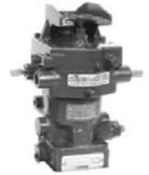
The **PSG governor** is a pressure compensated, speed-droop or isochronous governor for controlling the speed of small diesel, gas, and gasoline engines, or small steam or industrial gas turbines. The governor is used to control engines or turbines driving alternators, dc generators, pumps, or compressors.
