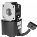
**The Flo-Tech™ ITB** integrated throttle body is designed for direct replacement of conventional throttle body with actuator and linkage. The throttle body will provide equivalent maximum flow rates of standard butterfly throttle bodies of the same diameter. The system contains a return spring to fully comply with DOT 571.124 specifications. The Flo-Tech integrated actuator/throttle body requires no actuator or linkage.
