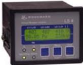
The **LS 4** is a power circuit breaker control for complex applications where additional section switches (such as bus-couplers) exist. The measurement value logging and the "switch-in-order" for the power circuit breakers are put into effect in the LS 4. The set value for the synchronization is transmitted from the LS 4 via the CAN bus to the genset controller (such as GCP).
