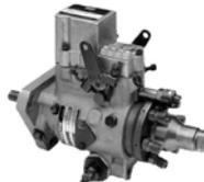
**The APECS® 70025 integrated actuator for Stanadyne "D" series injection pumps** is a proven all-electric, rotary actuator fully integrated into the cover of the Stanadyne pump. There are no brackets or external linkage, and the design is factory approved by Stanadyne. Installation is easy—simply remove the existing cover and install the new cover. Both a standard model and a completely sealed model are available.
