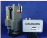
The **PGPL Actuator/Driver** is an electrohydraulic actuator with a proportional driver interface which can be used with electronic controls providing a 0 to 200 mA position signal. The actuator is designed for use with Woodward 2301A and D series, 700-series, Peak® 150, and 505 digital controls.
