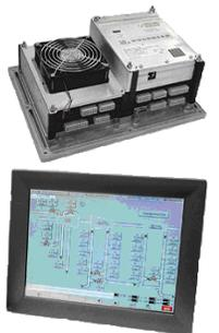
**The 505DE** is a microprocessor-based control with integral application software that is designed to control double automatic extraction/admission steam turbines. The turbine control architecture is patterned after the popular 505E Single Extraction/Admission Steam Turbine Control. Like the 505E, the 505DE uses configurable software for maximum field flexibility.
