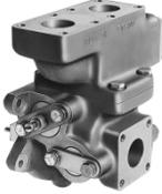
**The 1907 large liquid fuel valve** accurately meters liquid fuel to a gas turbine during acceleration, steady-state operation, and deceleration. The valve may be used for almost any liquid-fueled industrial gas turbine application within its range of fuel flow (70 to 340 kg/h; 150 to 25 000 lb/h). The 1907 valve is typically operated with a hydro-mechanical actuator.
