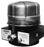
The Woodward **CPC Current to Pressure Converter** is designed for positioning steam and fuel valves and/or the associated servos. A 4–20 mA in/out signal is linearly and proportionally converted into a hydraulic output pressure. The CPC can thus interface with any electronic control, such as Woodward MicroNet™ systems and the Woodward 505 Control. It connects to pressure-operated servo systems and single-acting power cylinders. The CPC is suited for new as well as retrofit applications.
