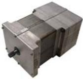
The **ProAct™ Digital Plus actuator** is intended to be mounted on-engine to control varying functions including (but not limited to): fuel rack positioning, timing control, throttle valve, and wastegate positioning. The actuator is effectively a positioner with an integral driver, which will accept a position command signal from another device in the system such as a speed control.
