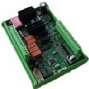
The **ST 2** Lambda Control is a digital Lambda control used to achieve low exhaust emission values in gas powered machines. The Lambda voltage is directly measured and evaluated in the ST 2. The regulating signals given to the gas regulating path may for instance be transmitted via a stepper motor or an analog output.
