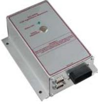
The **IC-100** is a microprocessor controlled, spark capacitive discharge ignition system capable of supplying ignition energy for a wide range of gas engines with 1 to 8 cylinders. The IC-100 is user programmable utilizing either RS-232 or CAN communications.
