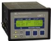
The **UMT 1** is a digital multi measuring transducer that measures true rms via three-phase measuring of voltage and current. Three analog outputs - 20/0/4→20 mA and an analog output manager offers the flexibility to output every measured and calculated value. The impulse output can be configured to output kWh/h or kVARh/h.
