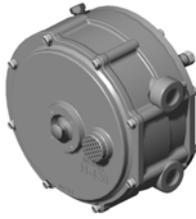
**Vapor Regulators / Vaporizer Regulators** offer improved vaporization. Liquid propane enters the regulator and then is vaporized using heat from the engine coolant. This is accomplished by spraying fuel against the regulator's thin heated walls. The diaphragm reacts to the fuel expansion due to vaporization, thus filling the expansion chamber and closing the high pressure valve.
