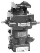
The **SG governor** hydraulic speed droop type governor is designed for use on small diesel, gas, or gasoline engines where isochronous control is not required. The design of the speed droop governor is such that the governor operates at a slower speed as engine load increases. It is through this characteristic that stability of the system is achieved and division of load between paralleled units is made possible.
