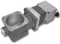
The ProAct™ ITB integrated throttle bodies are butterfly valves electrically-actuated by ProAct Analog and ProAct Digital Plus actuators to control flow output. With bore sizes of 105 mm, 120 mm, and 135 mm, these ProAct ITBs are designed for use with engines in the 1–2 MW range. The ProAct actuators are electro-magnetic, 75 degree-of-travel devices, and therefore alleviate the problems associated with linkages on gas engines (such as setup, non-linearity, and wear).
