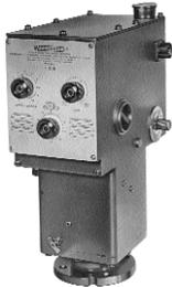
**The EGB Governor/Actuator** is used with Woodward analog or digital electronic controls that provide a proportional 20–160 mA signal to control dual fuel, diesel, and gasoline engines, and gas and steam turbines driving electrical or mechanical loads. The governor/actuator is available for outputs of 1, 2, 10, 13, 29, 35, 58, 200, and 300 ft-lb (1.4, 2.7, 14, 18, 39, 47, 79, 271, and 407 J) work capacity to position fuel racks or linkage.
