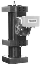
The **Electrohydraulic Power Cylinder (EHPC)** provides the force to operate the control valves of a steam turbine. The EHPC is intended for use on mechanical drives or generator driven turbines. The EHPC integrates the actuator, pilot valve, electronic feedback device, final driver and the power cylinder into a single package, eliminating linkage and reducing hydraulic plumbing and wiring.
