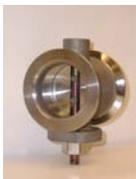
**The Glo-Tech™** modulating, all electric wastegate/bypass valve is capable of handling hot (600 °C) exhaust gasses for gas or diesel engines. The Glo-Tech valve provides engine manufacturers a method to reduce emissions, increase efficiency and reliability. The Glo-Tech valve has a bore of 60 mm and can accept an actuator case temperature of 100 °C.
