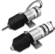
Woodward has numerous **solenoids**, both single-coil and dual-coil (allows the solenoid to remain energized for longer periods of time without overheating). Solenoids can be used to operate engine run/stop levers, throttles, chokes, valves, and clutches. They can also protect expensive diesel engines from overspeed, low lube pressure, and high temperature.
