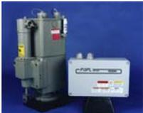
The PGPL Actuator/Driver is an electrohydraulic actuator with a proportional driver interface which can be used with electronic controls providing a 0 to 200 mA position signal. The actuator is designed for use with Woodward 2301A and D series, 700-series, Peak® 150, and 505 digital controls.
