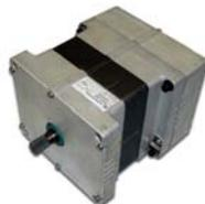
The **ProAct™ Integrated Speed Control (ISC)** is an electric actuator with an integrated electronic driver capable of diesel or gaseous engine speed control or positioning tasks. The ProAct ISC can be mounted on-engine to control a diesel fuel rack or gaseous throttle via linkage or integrated throttle body. The ProAct ISC accepts a speed input from an MPU and can accept a position command signal from another device in the system such as an engine control module.
