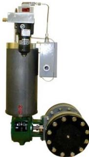
**The Woodward Gas Stop/Ratio Valve** performs a dual function for industrial or utility gas turbines. One function rapidly shuts off fuel to the turbine fuel control system. Another function provides accurate control of gas fuel pressure at the outlet of the stop/ratio valve. This pressure is applied to the inlets of the gas fuel control valve.
