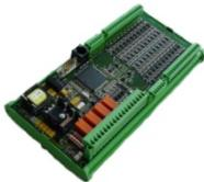
The **IKN 1** is an external 20 channel NiCrNi temperature scanner. It is an Intelligent Terminal NiCrNi to measure up to 20 different temperatures, including mean-value generation and limit-value monitoring. The measured data is transmitted via the CAN bus to the controller, where they can be displayed. Configuration via CAN bus is also possible.
