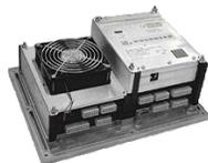
**The 505DE** is a microprocessor-based control with integral application software that is designed to control double automatic extraction/admission steam turbines. The turbine control architecture is patterned after the popular 505E Single Extraction/Admission Steam Turbine Control. Like the 505E, the 505DE uses configurable software for maximum field flexibility.
