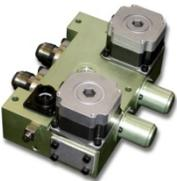
**Swift Gas Metering System**—The Swift Gas Metering System has been developed for microturbines, miniturbines, small industrial turbines (up to 2 MW), and high-pressure fuel cells. The Swift system has four valve sizes with maximum fuel flows between 6.3 and 88.9 g/s (50 and 695 lb/h) of standard natural gas, depending on system pressures. The system is designed for installation in the engine enclosure and can accommodate gas temperatures up to 121 °C (250 °F).
