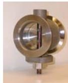
The **Glo-Tech™** modulating, all electric wastegate/bypass valve is capable of handling hot (600 °C) exhaust gasses for gas engines. The Glo-Tech valve provides engine manufacturers a method to reduce emissions, increase efficiency and reliability. The Glo-Tech valve has a bore of 60 mm and is typically coupled with a ProAct actuator
