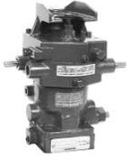
**The SG governor** hydraulic speed droop type governor is designed for use on small diesel, gas, or gasoline engines where isochronous control is not required. The design of the speed droop governor is such that the governor operates at a slower speed as engine load increases. It is through this characteristic that stability of the system is achieved and division of load between paralleled units is made possible.
