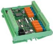
The **IKD 1** is an external I/O expansion board. If the digital inputs and outputs in the controller are not sufficient, 8 digital inputs and outputs can be connected via the CAN bus with this extension card. It is possible to connect two IKD 1 to the controller in parallel.
