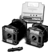
The **512/524 and 1712/1724 EPGs** are three-component governing systems for 12 or 24 Vdc operation. All EPG systems include an actuator, an electronic speed control, and magnetic pickup. Both isochronous and droop controls are available.
