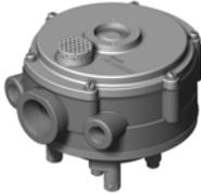
**The N-2000/N-2001 Vaporizer/Regulators** for LPG-fueled engines combines in a single compact unit the vital carburetion functions of a lockoff (fuel lock)/filter and a vaporizer/regulator. It eliminates the inefficient approach of an individual lockoff and vaporizer with their multiple hoses, fitting, electrical connections, and brackets.
