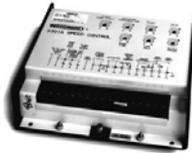
**The 2301A Speed Control** controls the speed or load of diesel or gas engines, or steam or gas turbines. The unit provides control in the isochronous mode, with droop available through an externally wired potentiometer. The isochronous mode is used for constant speed of the controlled prime mover as long as it is able to provide power to satisfy the load.
