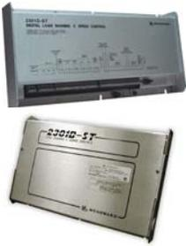
The **2301D-ST** is a microprocessor based control with integral application software designed for single-valve steam turbine applications. Like Woodward's 2301A line of controls, this control is housed in a sheet-metal chassis and consists of a single printed circuit board. To facilitate unit retrofits, the 2301D-ST's I/O terminals are located in the same general location as Woodward's 2301A line of controls.
