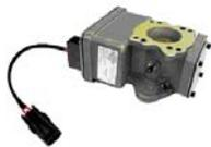
**The APECS® Power Flow integrated valve actuator** is designed for throttling the intake of internal combustion engines. The APECS Power Flow system is designed to couple to standard market-available fuel mixer series and to standard SAE flanged intake manifolds. This integrated throttle body is adaptable to a fuel injected engine for air control.
