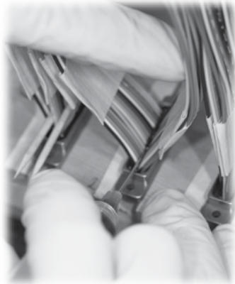
Potting a Micro-D with Epoxy-Filled Syringe
