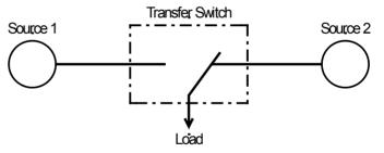
Figure 3-12: Open transition switch - connected to source 2
