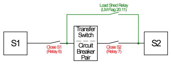
Figure 3-9: Load shed relay wiring - standard transition switch
