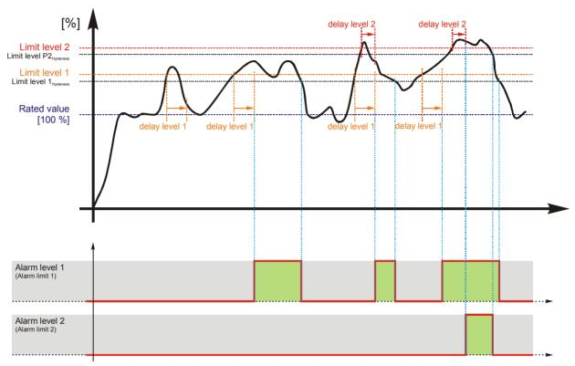
Figure 3-25: Monitoring - battery overvoltage
