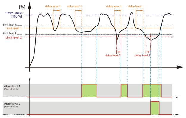
Figure 3-26: Monitoring - battery undervoltage
