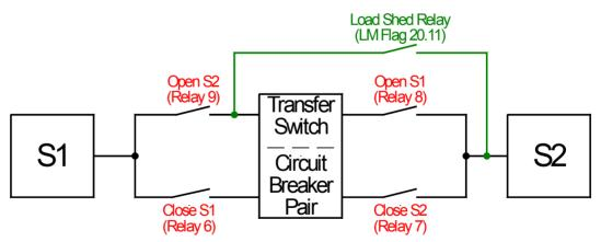
Figure 3-10: Load shed relay wiring - delayed or closed transition switch
