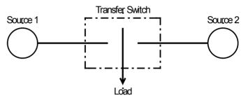
Figure 3-14: Delayed transition switch - neutral position
