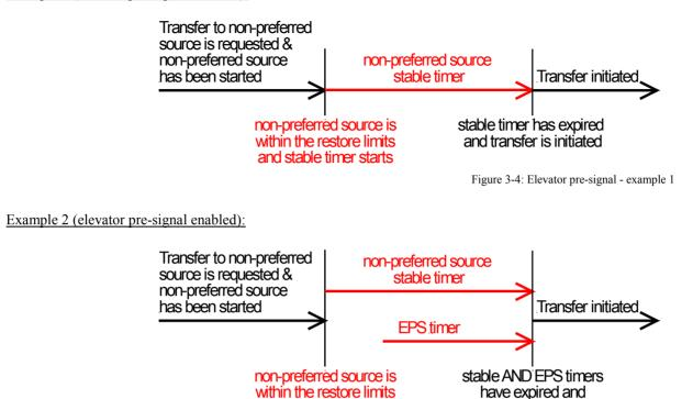
Figure 3-5: Elevator pre-signal - example 2
