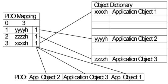
Figure 3-28: Interfaces - Principle of PDO mapping
