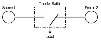
Figure 3-15: Delayed transition switch - connected to source 2
